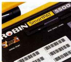
On-board Data Memory allows up to 1000 records to be stored
